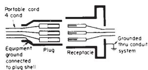
Typical 3-wire, 3-pole plug and receptacle
