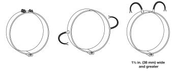
Expandable heaters are two-piece units with a common top metal that allow the heater to expand to the full diameter of the barrel. On expandable bands, each half will comprise one-half of the total wattage. On both expandable and two-piece bands, each half is rated at full operating voltage, unless otherwise specified.
