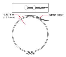
Two fiberglass lead wires exit a single, tightly woven metal braid at a right angle on the expandable construction vs. two sets of leads. The minimum diameter capability is 4 in. (102 mm). Minimum width capability is  $1\frac{1}{2}$  in. (38 mm). To order, specify **Type SLE** and **length.**
