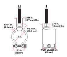
Type F: A loose fiberglass sleeving encloses two fiberglass leads for additional insulation protection where high temperature or minor abrasion is present. Leads are 2 in. (51 mm) longer than the sleeving. To order, specify **Type F** and **length**.
