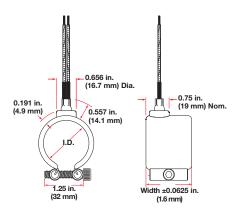
Type K: Flexible lead wires exit vertically from the heater. These leads can be bent adjacent to the heater for a quick and easy connection. To order, specify **Type K** and **length**.
