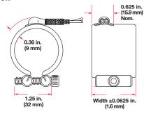
Leads Type B, Type B - 90° rotation, Type B - 180° rotation or Type C: Two fiberglass-insulated lead wires exit in a single metal braid providing good abrasion protection, lead flexibility and wiring convenience. Leads are 2 in. (51 mm) longer than the braid and are shipped with 12 in. (305 mm) leads, unless a longer length is specified. To order, specify **type** and **length**.
