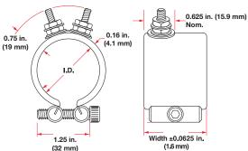
Post terminals provide optimum connections. The screw thread is 10-24. To order, specify **post terminals** (metric threads available).
