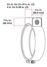
Metallic terminal boxes are available from stock on 3% in. inside diameter x 1% in. wide (89 mm x 38 mm) or larger heaters. Terminal boxes attach directly to the heater and act as a safety feature by covering the terminals. The conduit may be attached to the box through % in. (22.2 mm) diameter holes in the ends of the box. Two-piece heaters require two boxes. To order, specify **terminal box.**
