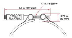
Welded barrel nuts with spring loaded clamping are used during start-up to maintain a tight heater fit on large barrels. This clamping variation is used for all MI band heaters greater than 14 in. (356 mm) in diameter and 1½ in. (38 mm) or greater in width. Refer to the MI Band Clamping Matrix Application Guide. For smaller diameter heaters, this is an option and must be ordered separately. To order, specify **spring loaded clamping.**
