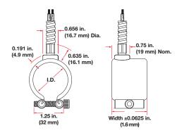
Type H: A flexible steel hose encloses the leads for maximum abrasion protection. Leads are 2 in. (51 mm) longer than the hose and are shipped with 12 in. (305 mm) leads, unless a longer length is specified. To order, specify **Type H** and **length.**
