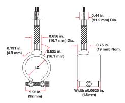
Type E: A loose metal braid encloses two fiberglass leads to provide good abrasion protection, lead flexibility and wiring convenience. Leads are 2 in. (51 mm) longer than the braid and are shipped with 12 in. (305 mm) leads, unless a longer length is specified. To order, specify **Type E** and **length**.
