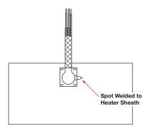
ASTM Type J or K thermocouples are available on lead Type B with loose braid and fiberglass sleeving. They are also available on E, F and H leads. The thermocouple junction, spot-welded to the heater sheath, provides a signal for measuring relative heater temperature. A separate thermocouple is available.
