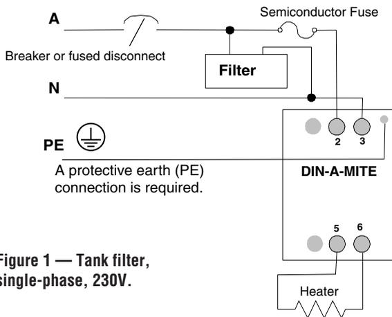
Figure 1 — Tank filter, single-phase, 230V.
