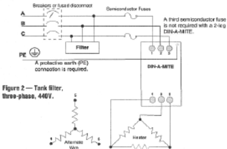
**Figure 2 — Tank filter, three-phase, 440V.**
