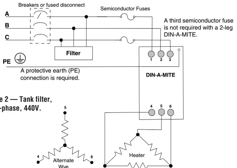
Figure 2 — Tank filter, three-phase, 440V.
