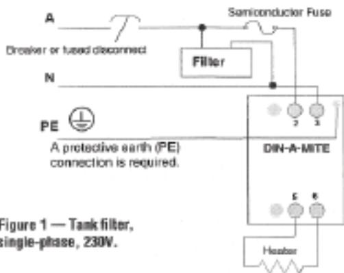
**Figure 1 — Tank filter, single-phase, 230V.**
