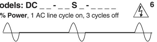
**50% Power, 1 AC line cycle on, 1 cycle off**
