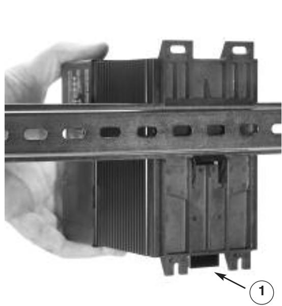
1. Press down on the release tab while rotating the unit up and away from the rail.
