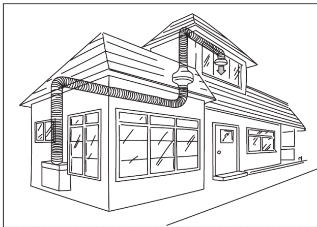
(TURBO Fan) transferring conditioned air to a new room addition
