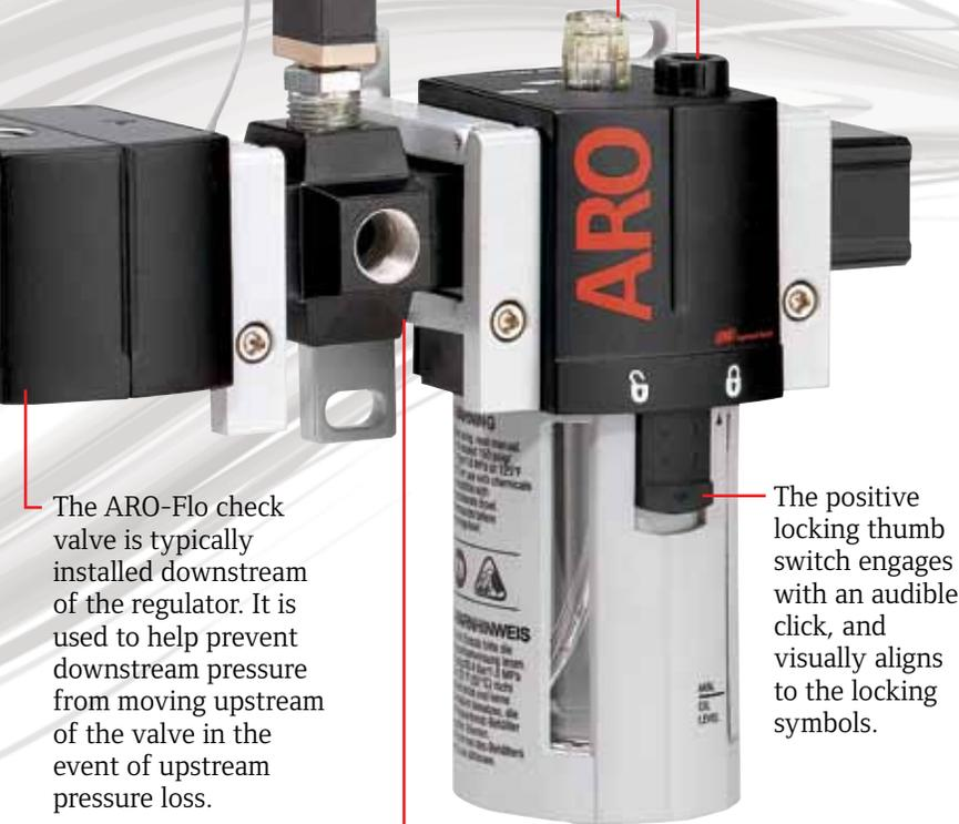
The ARO-Flo check valve is typically installed downstream of the regulator. It is used to help prevent downstream pressure from moving upstream of the valve in the event of upstream pressure loss.
