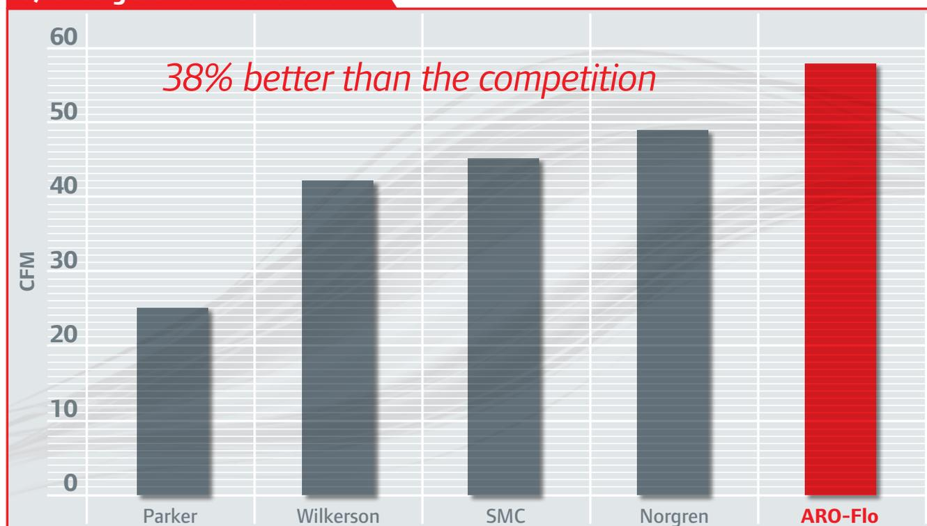
Test parameters: 100 psi inlet pressure, 90 psi set pressure, and 33 psi drop
