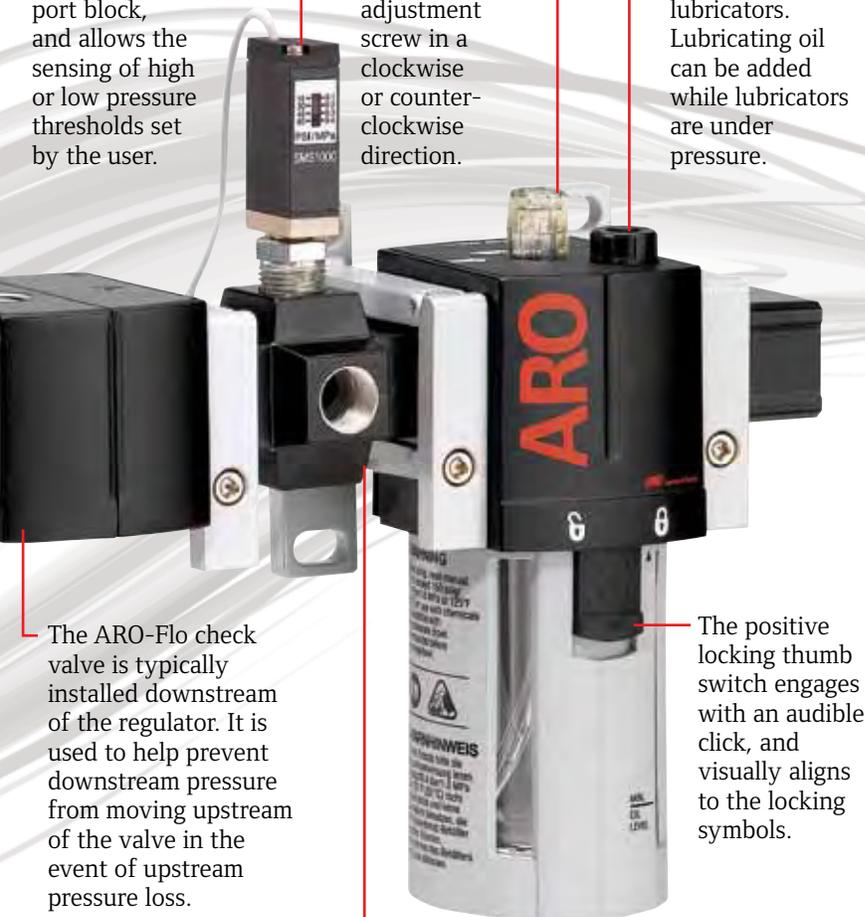
The ARO-Flo check valve is typically installed downstream of the regulator. It is used to help prevent downstream pressure from moving upstream of the valve in the event of upstream pressure loss.
