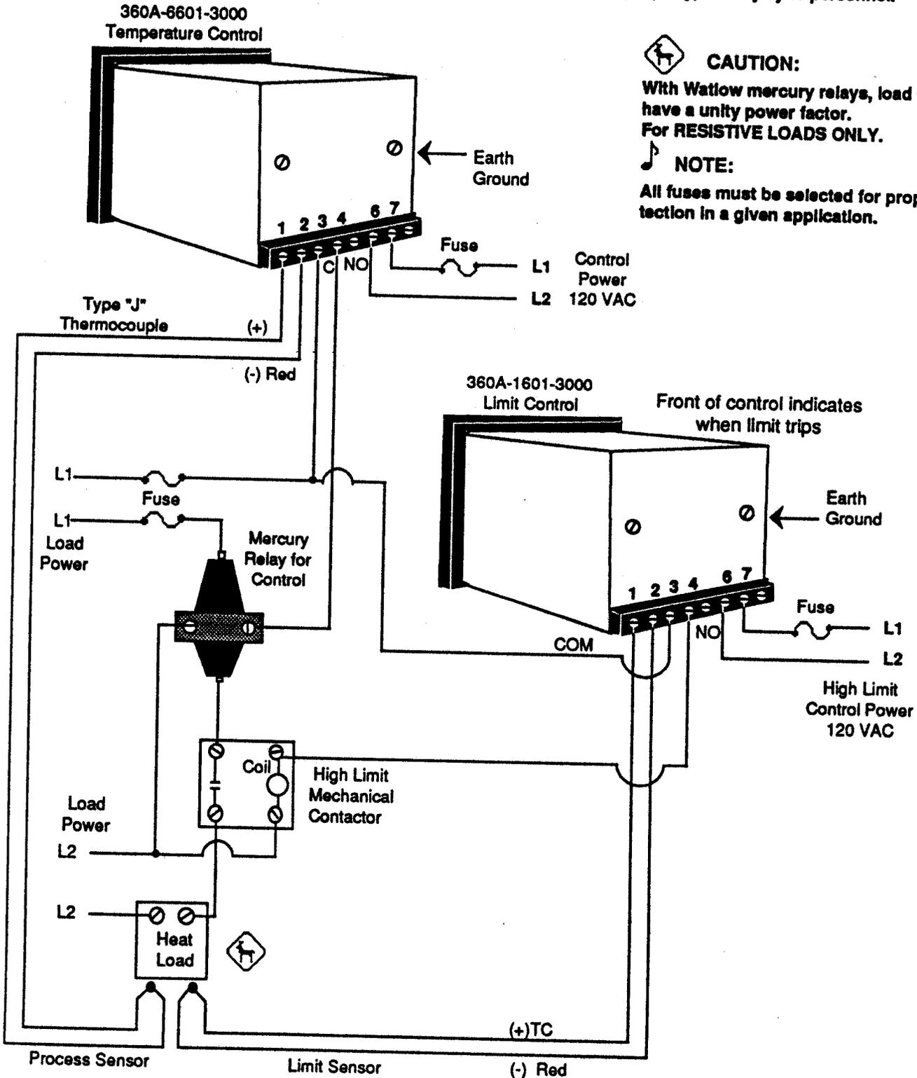
Figure 10 - Series 360 System Wiring Example
