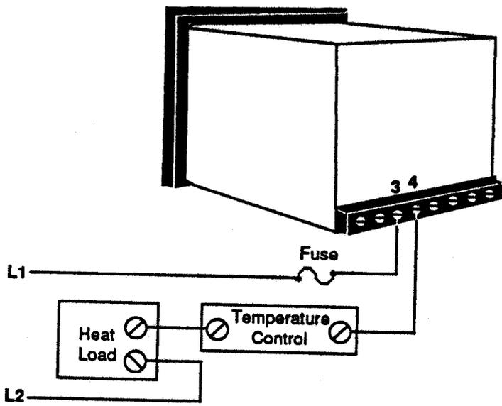
Figure 8 - Limit Output Wiring (360A-[1,3]XXX-X000)
