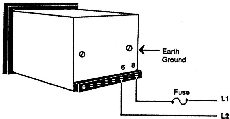
Figure 6- 240 VAC Power Wiring (360A-XXXX-3000)
