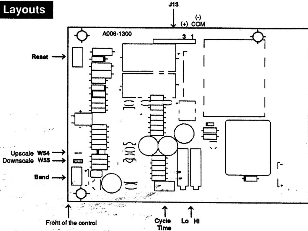
Figure 11 - A007-1300 Limit/ON/OFF Board
