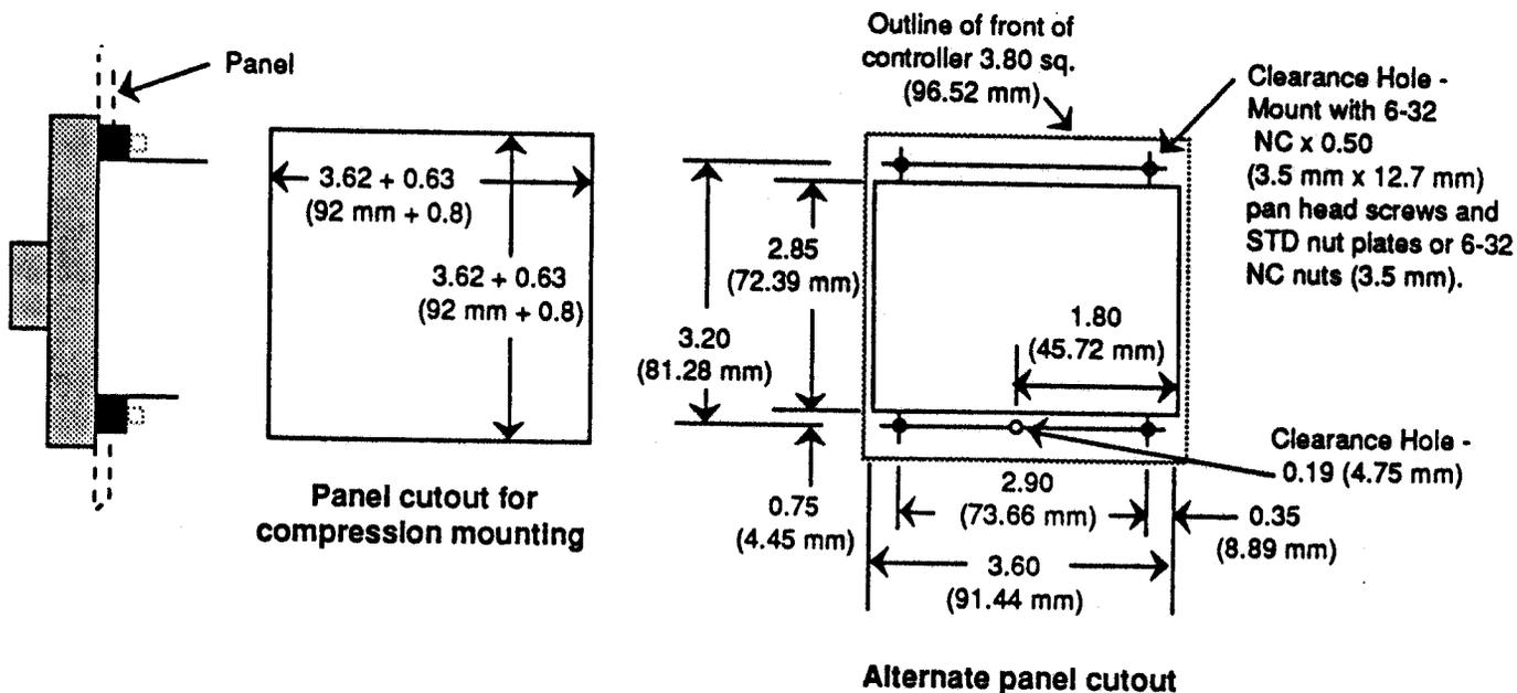
Figure 2 - Mounting Requirements
