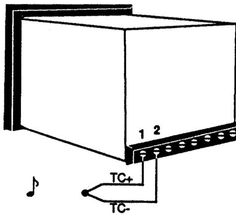
Figure 7 - Thermocouple Input (360A-XXXX-X000)
