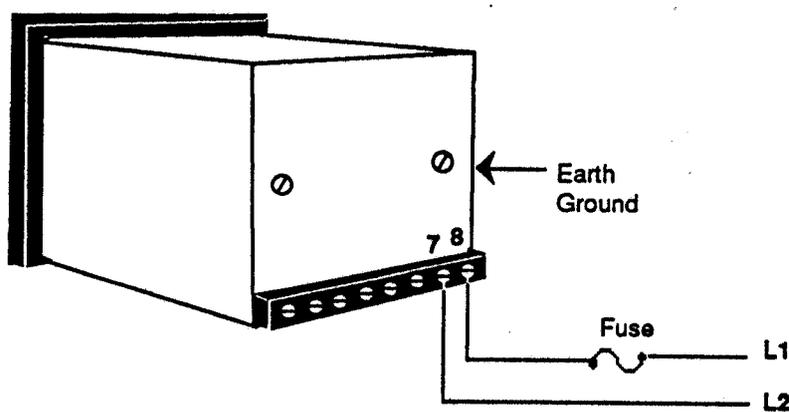
Figure 4- 240 VAC Power Wiring (360A-XXXX-2000)
