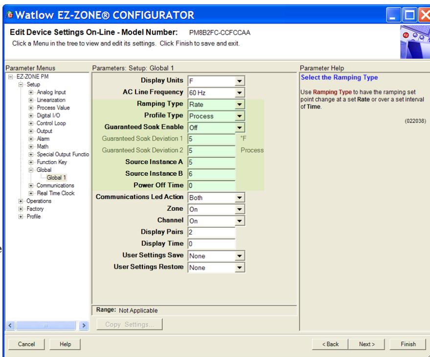
Once these global profile features are configured, the next step will require navigation to the Profiling Page. Here, each desired ramp and soak profile will be configured.
