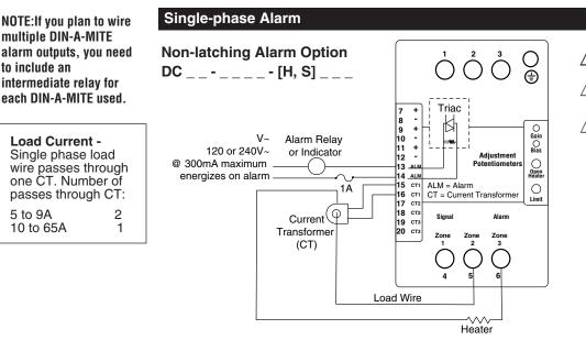
The Watlow DIN-A-MITE alarm option provides a common alarm output for open-heater or shorted SCR conditions. **This is a non-latching alarm.**
