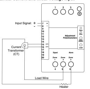
The Zone 3 indicator light serves as the current-limit indicator in phase-angle, current-limit models.
