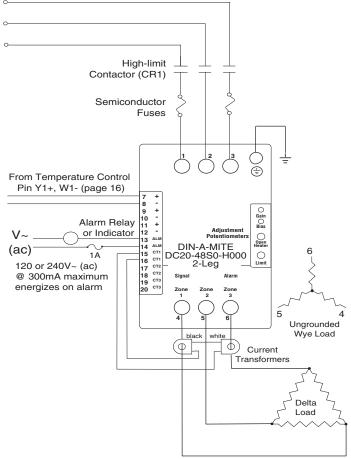
Non-latching Alarm Option (models DC\_\_-S\_-H\_\_\_)
