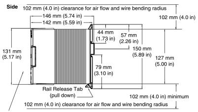
Front panel is touch-safe, no clearance is required.
