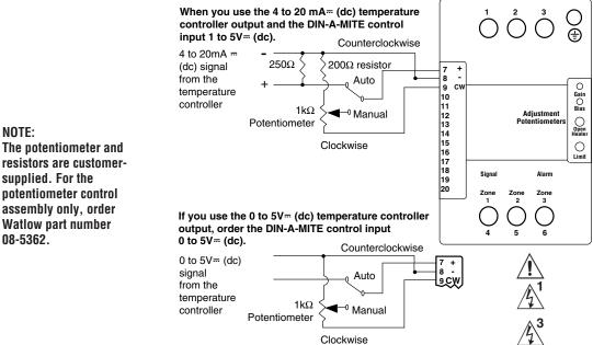
NOTE: The potentiometer and resistors are customersupplied. For the potentiometer control assembly only, order
