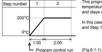
This program pattern shows that the temperature rises to  $200^{\circ}$ C for 1 hour and stays at  $200^{\circ}$ C for 2 hours.
