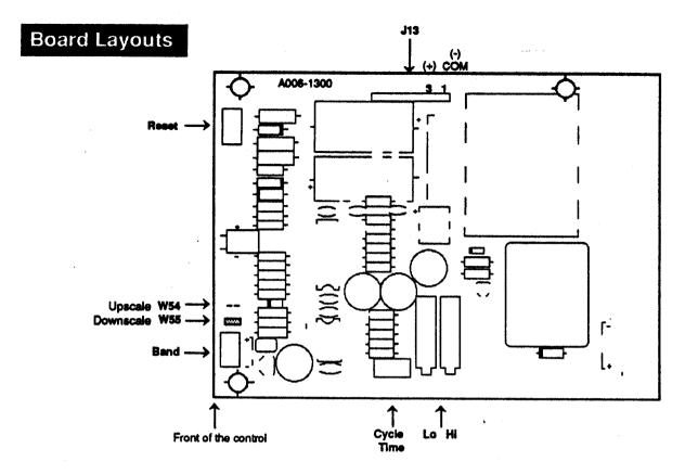
Figure 11 - A007-1300 Limit/ON/OFF Board
