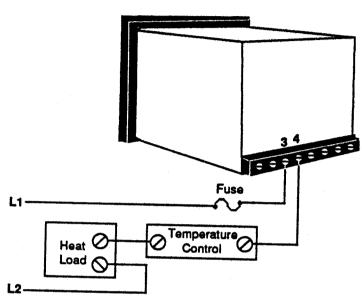
Figure 8 - Limit Output Wiring (360A-[1,3]XXX-X000)
