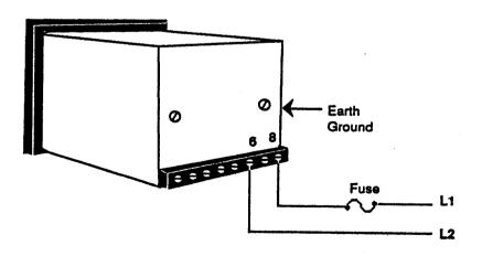
Figure 6- 240 VAC Power Wiring (360A-XXXX-3000)
