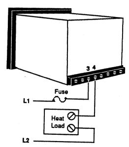
Figure 9 - Time Proportioning or ON/OFF Output Wiring (360A-[5, 6]XXX-X000)
