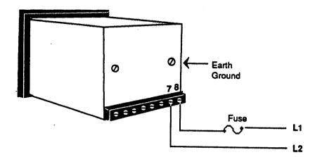
Figure 3 - 120 VAC Power Wiring (360A-XXXX-1000)
