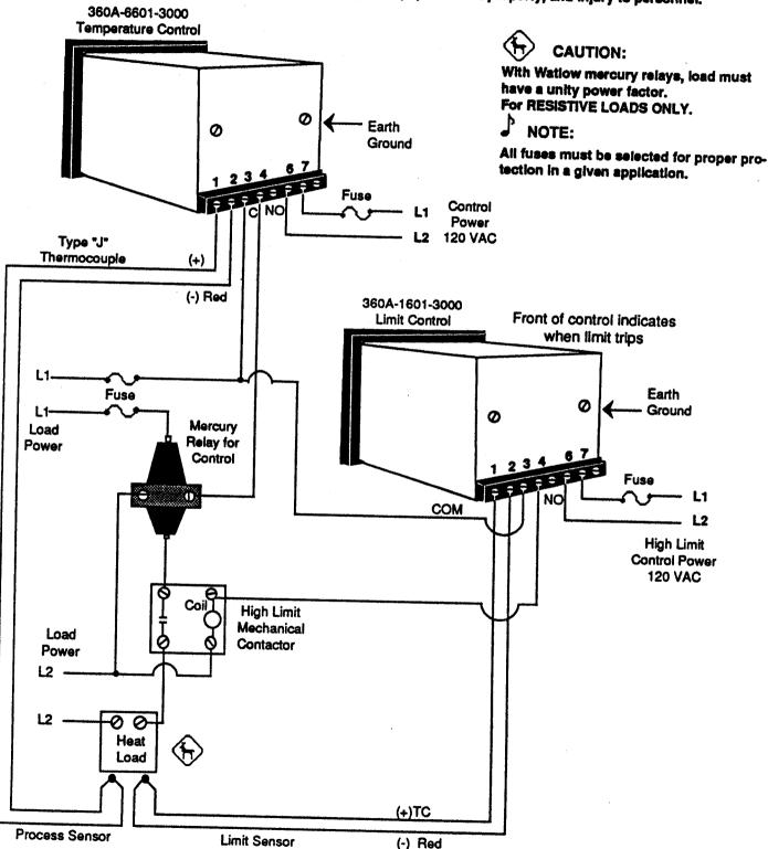
Figure 10 - Series 360 System Wiring Example
