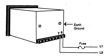
Figure 4- 240 VAC Power Wiring (360A-XXXX-2000)
