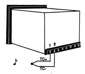
Figure 7 - Thermocouple Input (360A-XXXX-X000)
