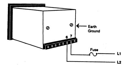
Figure 5 - 120 VAC Power Wiring (360A-XXXX-3000)
