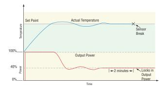
Input Error Latching (Setup Page, Analog Input Menu) determines the controller's response once a valid input signal returns to the controller. If latching is on, then the controller will continue to indicate an input error until the error is cleared. To clear a latched alarm, press the Advance Key (Hendrick) the Up Key (D.
