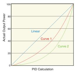
Select a nonlinear cool output curve with Cool Output Curve **[[]** (Setup Menu, Loop Menu).
