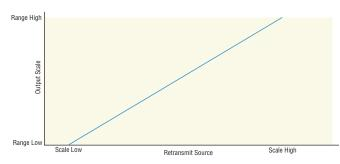
Set the range of the process output with Scale Low 5.6 o and Scale High 5.6 i. Scale the retransmit source to the process output with Range Low r.6 o and Range High r.6 i.
