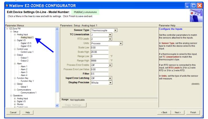
In the screen shot above notice that the device part number is clearly displayed at the top of the page (green highlight added for emphasis). When multiple EZ-ZONE devices are on the network it is important that the part number be noted prior to configuring so as to avoid making unwanted configuration changes to another control.
