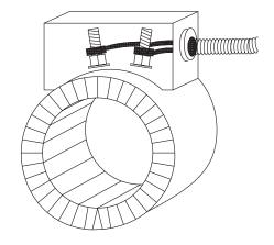
Flexible stainless steel hose is welded to the terminal box with a coupler. This terminal option provides superior mechanical protection where lead abrasion is a problem. Leads are attached to posts with a ring connectors.
