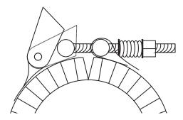
Latch and trunion clamps provide a quick clamp option. Clamping force is similar to barrel clamps and a spring is included to allow for thermal expansion of metals.
