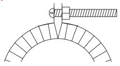
Clamp tabs are a standard clamping option that offers a uniform clamping force across the heater width.
