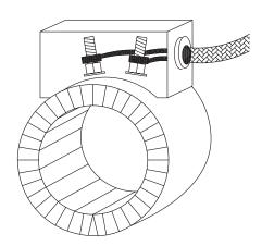
The stainless steel braid method includes a loose metal braid that is welded to the terminal box with a coupler. This provides excellent abrasion protection and flexibility. Leads are attached to posts with a ring connector.
