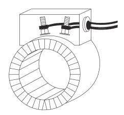
Flexible lead wire exits tangential to heater and includes leads connected to the post terminals with ring connectors. This termination method requires a terminal box.
