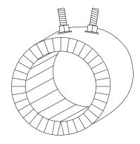
Post terminals are the standard termination, providing quick connection with ring or fork connectors or buss strips, ¼ -20 in. thread and includes double nuts and washers. Standard terminal location is 180° from gap.
