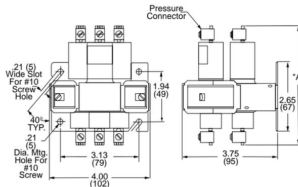
**⚠ WARNING:** Mercury displacement relay must be mounted vertically. Failure to do this will prevent the contacts from turning off, which will supply full voltage to the load. Failure to follow this guideline could result in damage to equipment, and personal injury or death.
