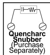
**Note:** Watlow temperature control solid state outputs will not drive VDC coils directly. Refer to the coil current specifications above and any temperature control output specifications as required by the application.
