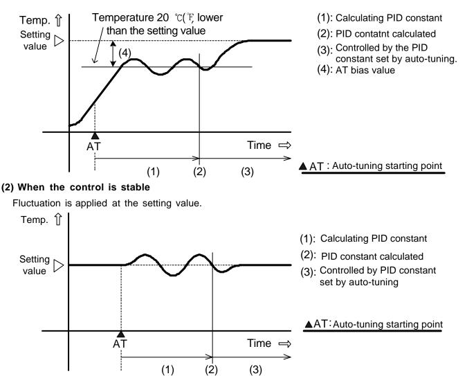
(3) When the difference between the setting value and processing temperature is large as the temperature falls.
