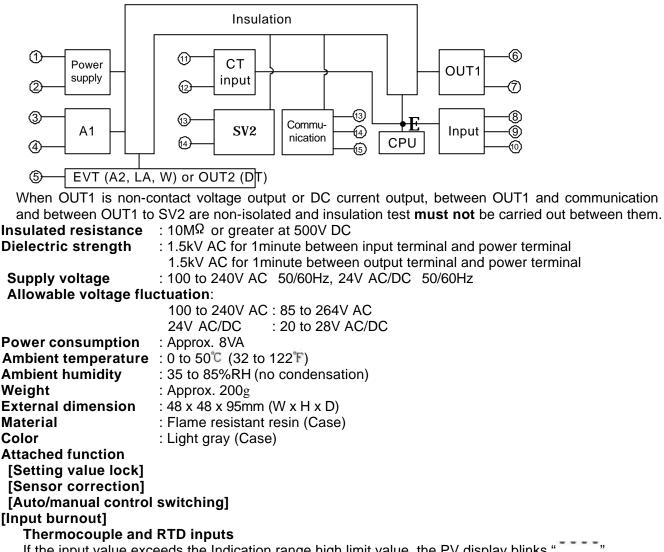
If the input value exceeds the Indication range high limit value, the PV display blinks """, and if the input value exceeds the Indication range low limit value, the PV display blinks "2222". If the input value exceeds the Control range, OUT1 and OUT2 are turned off (for DC current output type, OUT1 low limit value and OUT2 low limit value).
