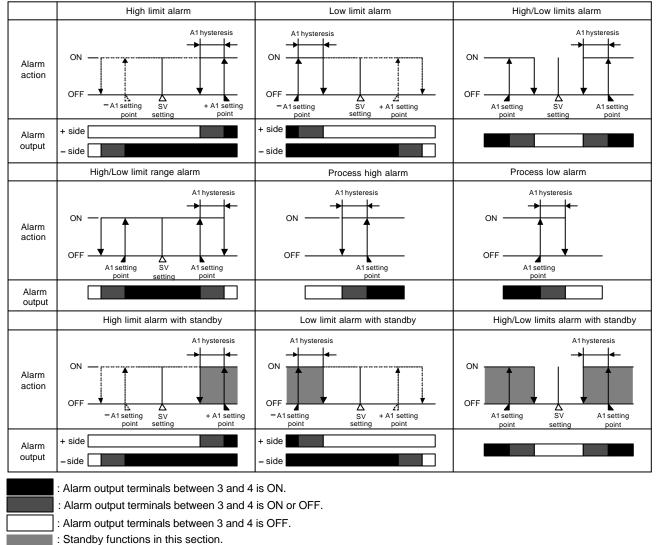
A1 indicator lights up when output terminals between 3 and 4 is ON, and goes out when between them is OFF.
