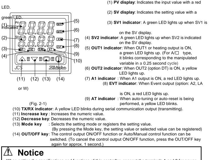
When setting the specifications and functions of this controller, connect the terminals 1 and 2 for power source first, then set them referring to "5. Setup" before performing "3. Mounting to control panel" and "4. Wiring connection".
